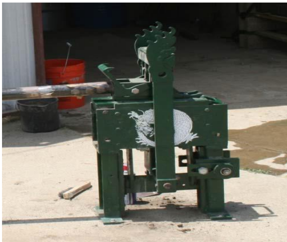
Figure: Sheng Thai BP6 Block press
